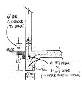
Accessory buildings smaller than 400 sq. ft. may be installed with monolithic slab.
